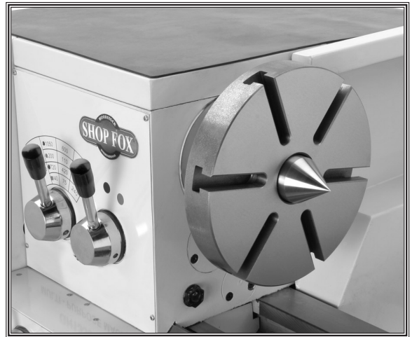
Figure 31. Faceplate and dead center setup.
